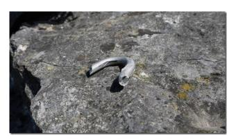
The load at deformation was consistent within a range of 11-15kN giving a mean of 13.28kN.
